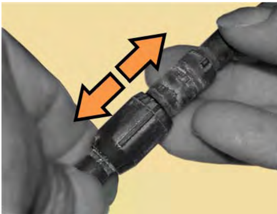
Figure B-16. Disconnect the Fan 1 / Fan 2 Power Supplies
