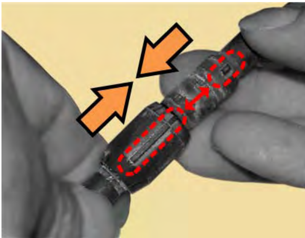
Figure B-18. Reconnect the Fan 1 / Fan 2 Power Supplies
