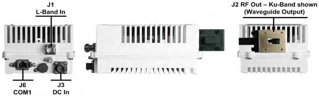
Figure 2-1. LPOD-R PS .5 Connectors
