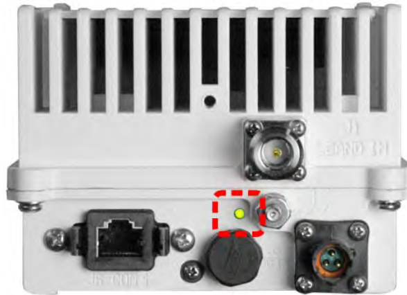
Figure 2-13. LPOD-R PS .5 LED Indicator
