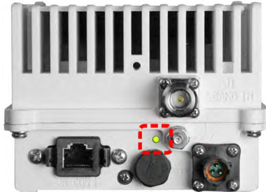
Figure 1-3. LPOD-R PS .5 LED Indicator
